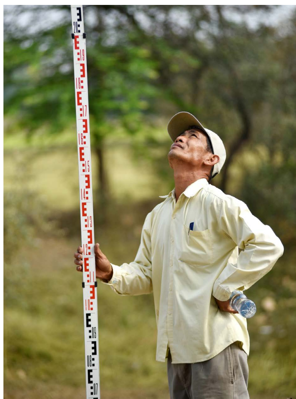
In Cambodia , ActionAid's partner Ockenden has worked with communities to install water gauges that will help monitor water levels and the likelihood of floods.
